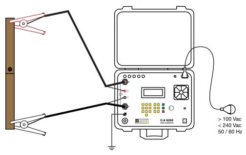
Tighten the terminals well to reduce the contact resistances and limit heating. Make sure that the leads are correctly uncoiled and do not form loops.
